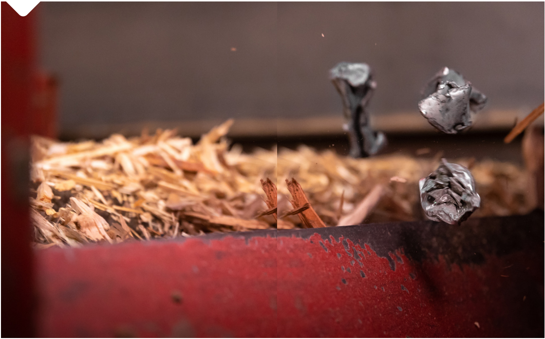
Metal detection and separation at waste wood sorting line. The recycled wood is used in panel manufacturing, Commercial Waste NL, Nieuwegein
